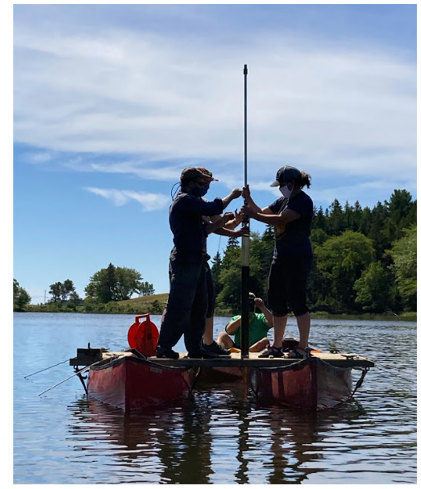
Fig. 1: Core extraction with a Livingston Piston 2" barrel
